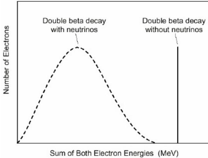
Figure 6: The energy spectrum of the sum of the energies of the emitted electrons for  $2\nu$  double beta decay (broad continuous distribution) and  $0\nu$  double beta decay (spike at endpoint of the spectrum).
