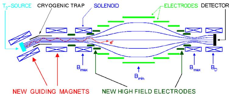
Figure 3: Schematic of a tritium-beta decay experiment.
