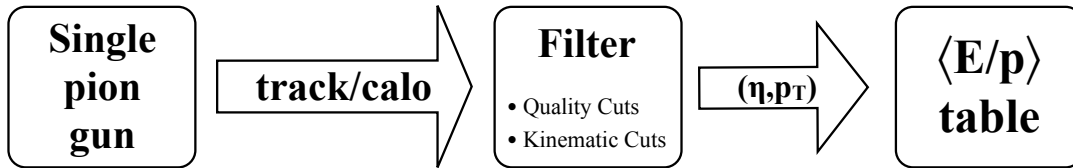
Figure 2: Conceptual process used to derive the calorimeter response function starting with a single \pi sample.
